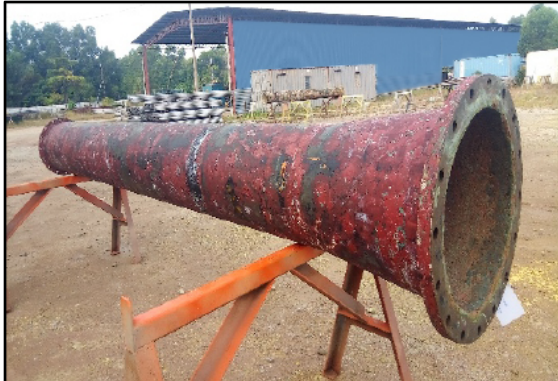
Pipe section after hot water pressure wash.
